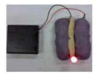
the LED but be sure that the short end of the LED is inserted into the same piece of conductive dough that holds the black, or negative, battery pack wire. It is good practice to turn the battery pack off while you are connecting the components and to turn it on after you have finished setting up the circuit.
