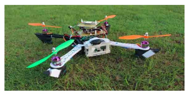
In this project, you can see a quadrotor, which has been built using a raspberry pi. The system uses IMU sensors and brushless motors for stabilizing and powering the copter. Check out the video:
